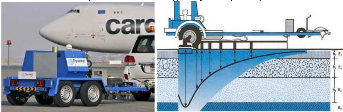
Figure 1 Typical HWD and this application on pavements
